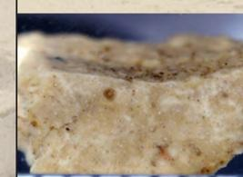
Plaster section from headboard region of (40106) box coffin. Lime and gypsum were not burnt hot enough to produce an effective mortar.
