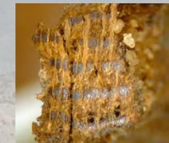
Sycomore: diffuse-porous vessel distribution and regular alternation of parenchyma and fibre bands, which create distinct colour streaks.
