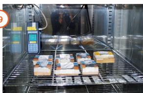
9. Artificial aging: thermo-hygrometric variation (T 16°C RH 60% for 15 minutes; T 35°C RH 70% for 99 minutes; T 35°C RH 75% for 99 minutes; T 15°C UR 60% for 10 minutes)
