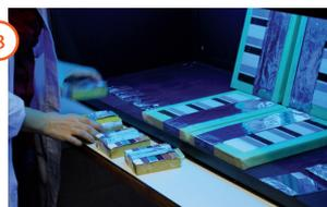
8. Artificial aging: UV radiation. Constant temperature and relative humidity (T 26°C RH 50%)
