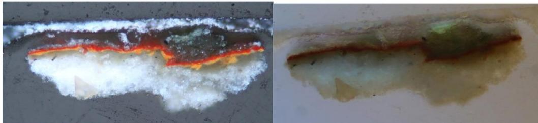
Figure 5: E.1.1822 Cross section OB23 (interior, Green – inside figure's decoration), 20x, visible light (left), ultraviolet light (right).
