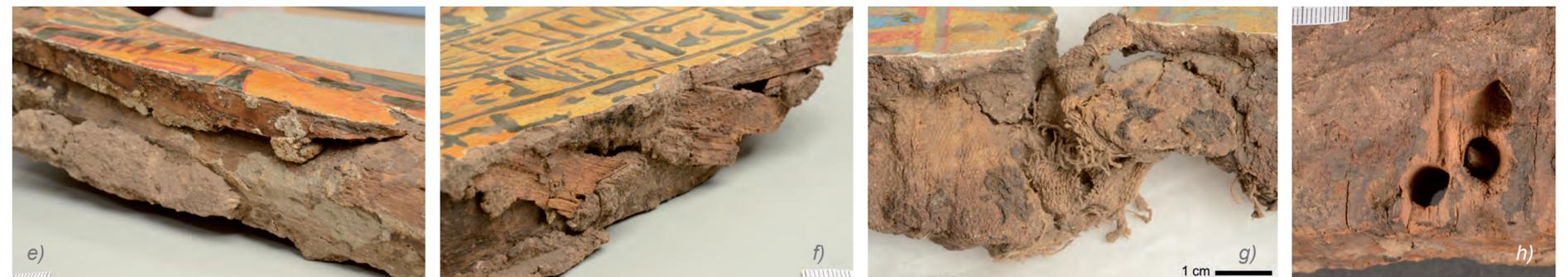
Fig. 2 e-h e, f and b) Small wooden wedges with animal glue and filling mass; g) textile (flax) as filling material; h) cubically shaped holes for dowels 8-10 mm.
